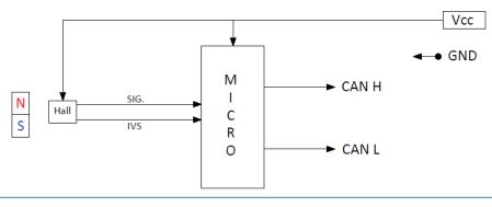
CAN message can be electronically configured in accordance with motor's specific requirements.
